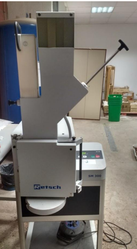
Retsch/ cutting mill 3 kW, 1500 rpm
